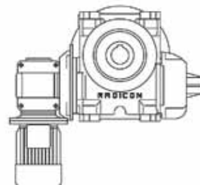
Motorized Double Reduction Units (worm/worm)
